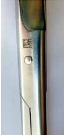
Figure 2. Coding the surgical instrument
